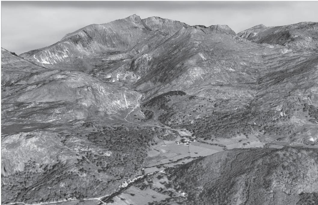
**Figure 6.27** The image is a three-dimensional visualization of an area in northern Wales U.K. A color air-photo has been merged with the STAR-3i DSM and presented as a perspective view or 'hill-shade'. The air-photo was supplied by GetMapping plc. Figure courtesy of Intermap Technologies Inc. See color plate in Appendix C.
