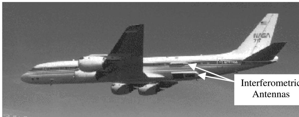
**Figure 6.18** View of the NASA DC-8 in flight with the AIRSAR and TOPSAR antennas clearly visible where they are mounted on the fuselage. See color plate in Appendix C.
