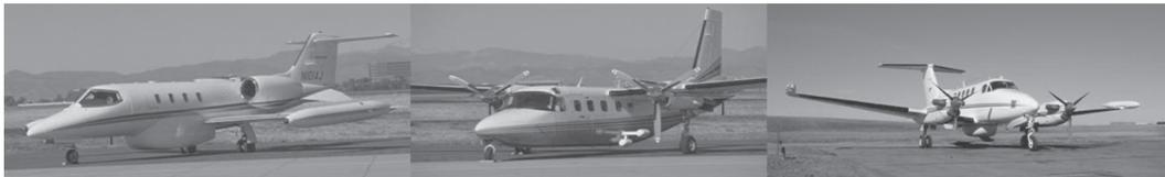
**Figure 6.25** The three images show the STAR-3i, TopoSAR and STAR-4 platforms respectively. TopoSAR is the only system with antennas not enclosed within a radome. Figure courtesy of Intermap Technologies Inc. See color plate in Appendix C.
