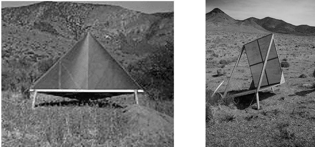
**Figure 6.41** The two types of corner reflectors normally deployed for SAR calibration are a trihedral shown in the left of the figure and a dihedral shown in the right of the figure. Physical size of a corner reflector used for calibration is a function of the wavelength, radar transmit power, antenna size and range. The trihedral in this figure is approximately 2.6 m measured along a diagonal edge and the dihedral is about 2 m high.
